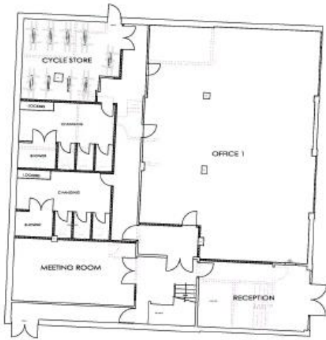
GROUND FLOOR PLAN SCALE 1:100
